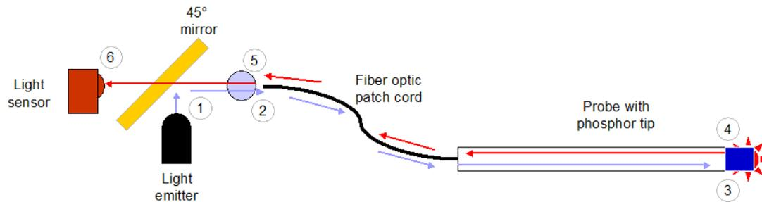
**Figure 2 - Conceptual representation of temperature sensing using the fluorescence decay principle**
