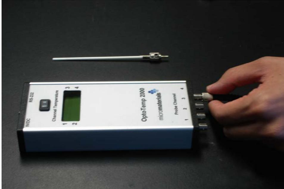
2. Remove probe from packaging and attach to the other end of the patch cord using the fiber optic mating sleeve.
